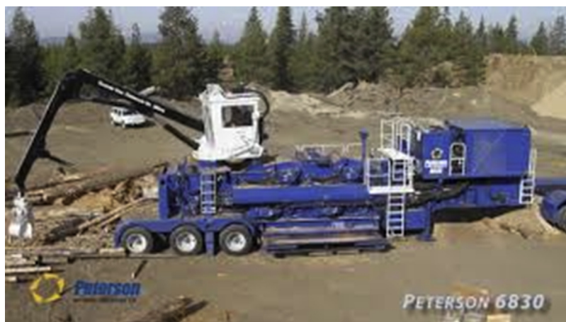
FIGURE 11.15 Disc Chipper from Peterson. Courtesy Peterson Pacific Corp. and Michael Spreadbury (photographer).
