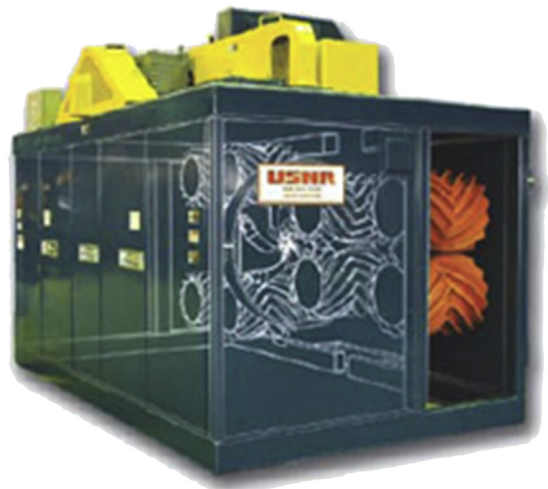
FIGURE 11.7 Ring debarker (USNR). Courtesy of Logging and Sawmilling Journal, www.forestnet.com .
