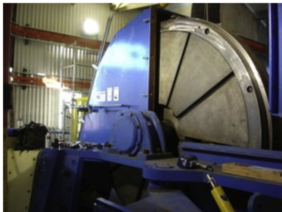
FIGURE 11.11A Whole log chippers. Courtesy of Acrowood.
