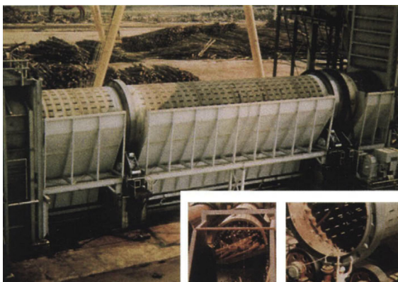
PLATE 2.4 Barking drum 14.5 ft in diameter by 100 ft long. The first insert shows the logs at the dam, and the second insert shows the inside of the drum during construction. Courtesy of Manitowoc Engineering Co. Ring barker with an insert of a modular, rotary-head option to debark stringy-bark species such as cedar and eucalyptus; Courtesy of Valon Kone Brunette, Ltd.
