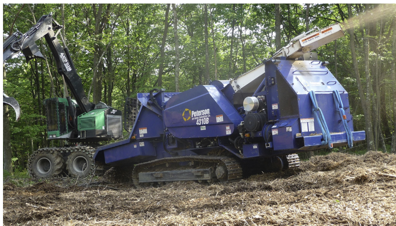
FIGURE 11.13 Drum chipper P1020314 from Peterson. Courtesy Peterson Pacific Corp. and Michael Spreadbury (photographer).
