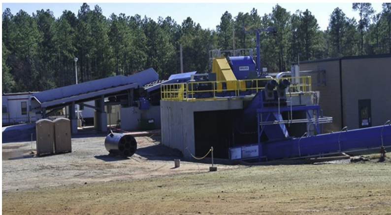
FIGURE 11.12 Drum chippers 4310B from Peterson. Courtesy Peterson Pacific Corp. and Michael Spreadbury (photographer).
