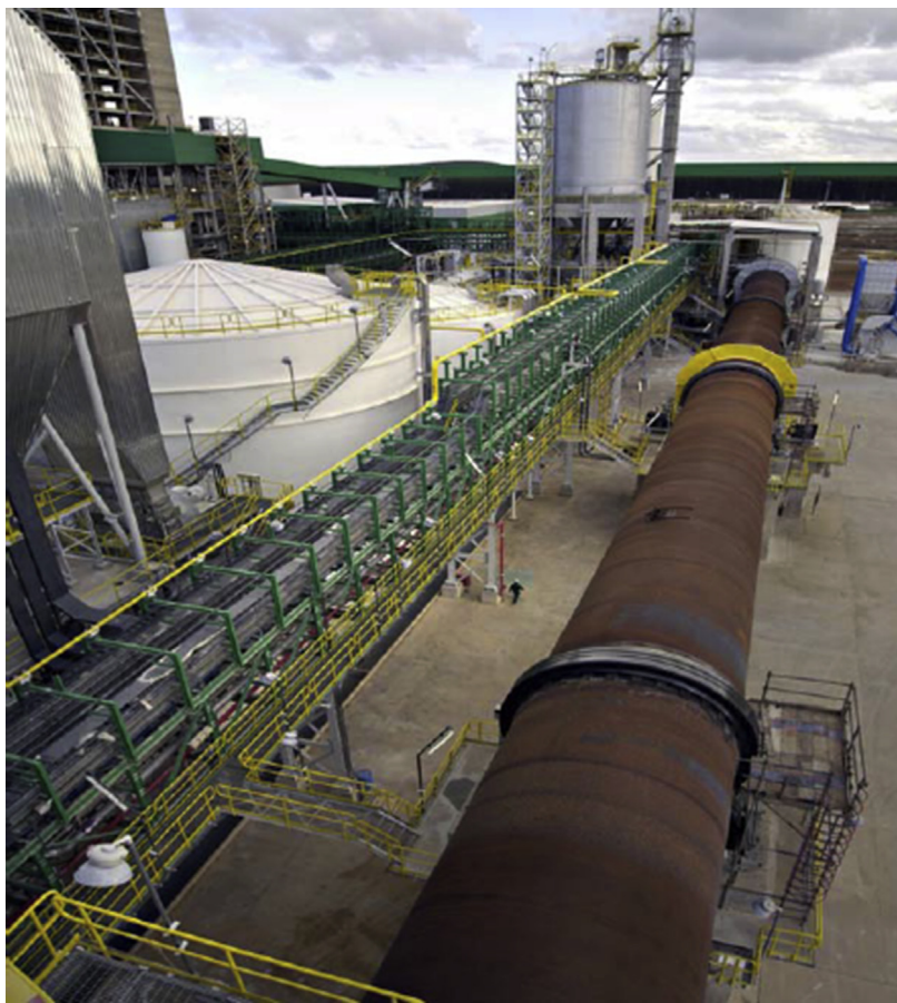
FIGURE 17.18 Andritz's lime reburning kiln system ensures reliable and energy efficient production of high-quality lime for the recausticizing operation. Courtesy: Andritz
