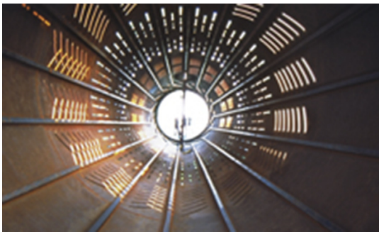
FIGURE 11.4 Andritz debarking drum. Courtesy of Andritz.
