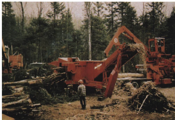
PLATE 2.6 Flail barker. Courtesy of Manitowoc Engineering Co.
