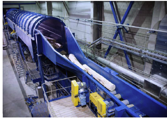
FIGURE 11.5 Andritz Rotary debarker RotaBarker. Courtesy of Andritz.
