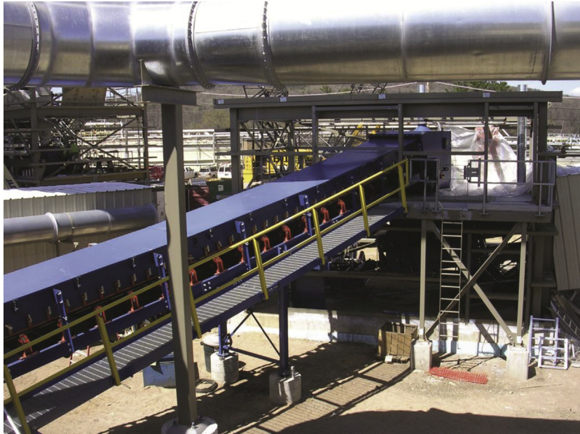
FIGURE 11.19 Belt conveyor. Courtesy FEECO International, Inc. — Process Development & Equipment Manufacturing — Green Bay, WI USA.
