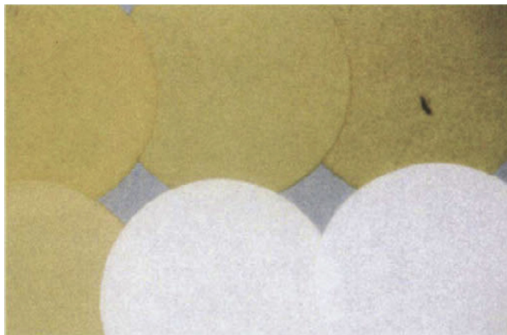
PLATE 19.1 Handsheets at various stages of bleaching. From upper right, counterclockwise the pulp samples are (1) unscreened, (2) screened, (3) after chlorination, (4) after alkali extraction, (5) after hypochlorite treatment, and (6) after hydrogen peroxide bleaching.
