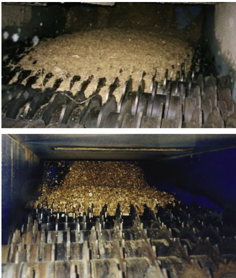
FIGURE 11.17 Disc screens. Courtesy of Advanced Biomass Consulting Inc., Canada; http://www.advancedbiomass.com/2014/10/disc-screen-fundamentals/ .
