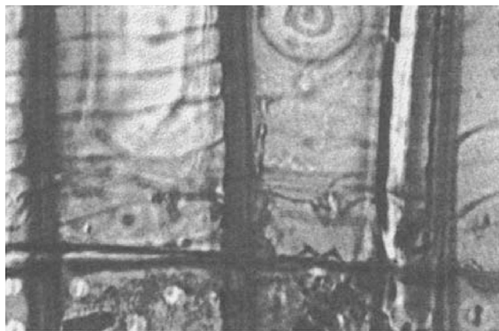
FIGURE 4.12 Spiral thickening in Douglas fir tracheids, approximately 600 \times .
