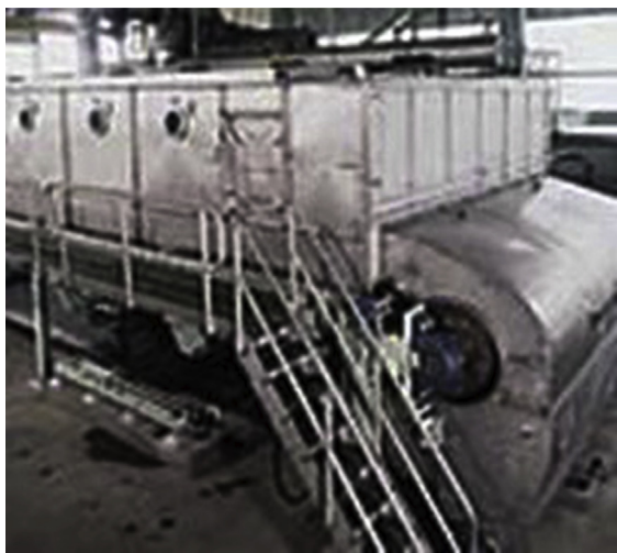
FIGURE 15.9 Kadant Black Clawson Chemi-Washer. Courtesy Kadant.
