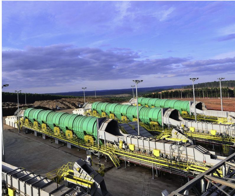
FIGURE 11.2B Andritz debarking process. Courtesy of Andritz.
