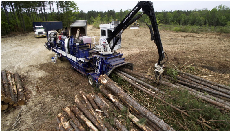
FIGURE 11.11B Whole tree chipper. Courtesy Peterson Pacific Corp. and Michael Spreadbury (photographer).
