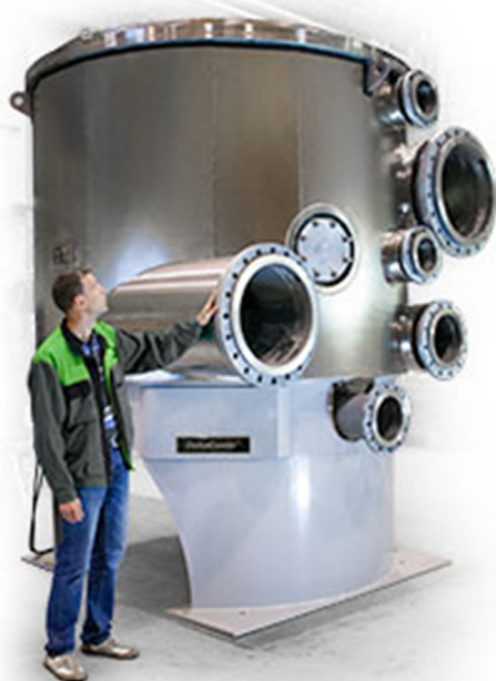
FIGURE 16.8 DeltaCombi (combines knoter and fine screen). Courtesy Valmet.
